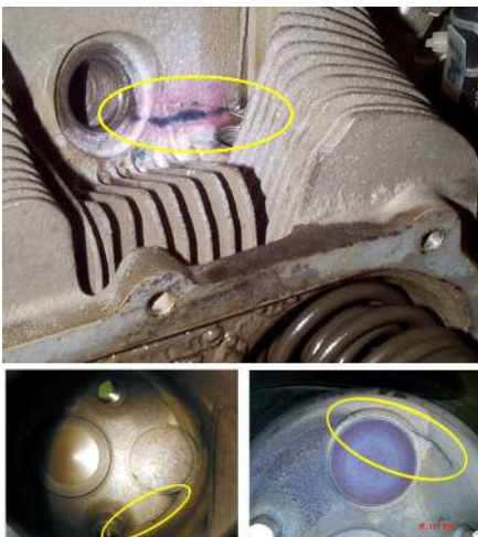
Caption: Figure 2— Cylinder head cracks are very common, and roughly 99.9% of them are benign.
