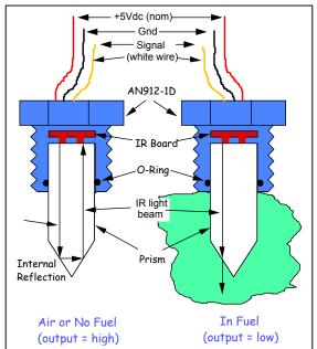
detector senses fuel or air.) When the FSD is installed near the bottom of a fuel tank, a "high" signal from the detector signals a near-empty fuel state. When the FSD is installed near the top of a fuel tank, a "low" signal indicates a near-full fuel state. Alternatively, the output of the FSD detector may be used to illuminate a lamp or provide other similar functions; the use is limited by the 100mA maximum current draw of the FSD circuit.
