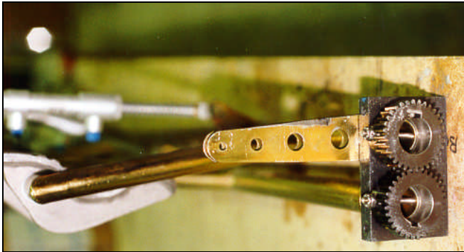
Spurgears ganging rudder pedal tubes (both ends)
