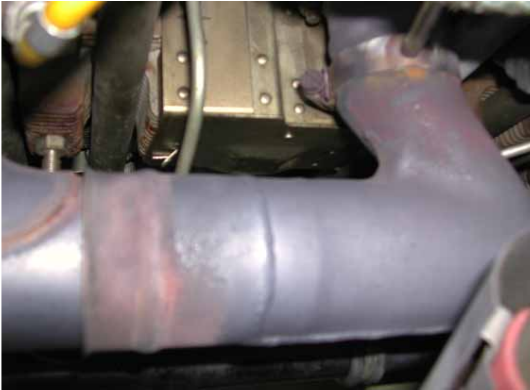
Lancair inter-cylinder duct very similar to Cirrus below.
