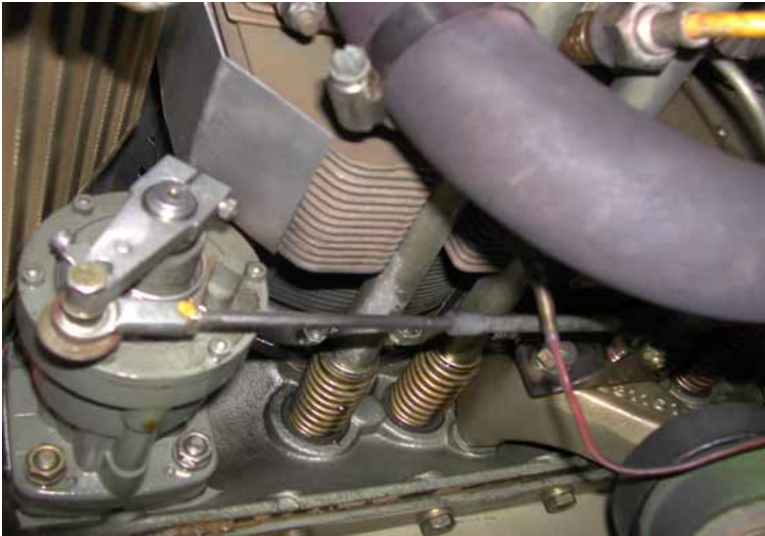
Lancair forward cylinder pilot side. This should cover fins and have sides.
