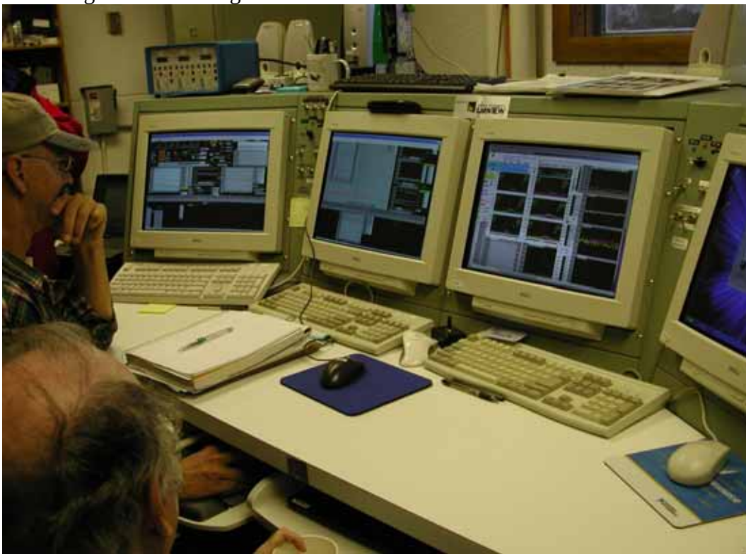
Engine test operator consoles.
