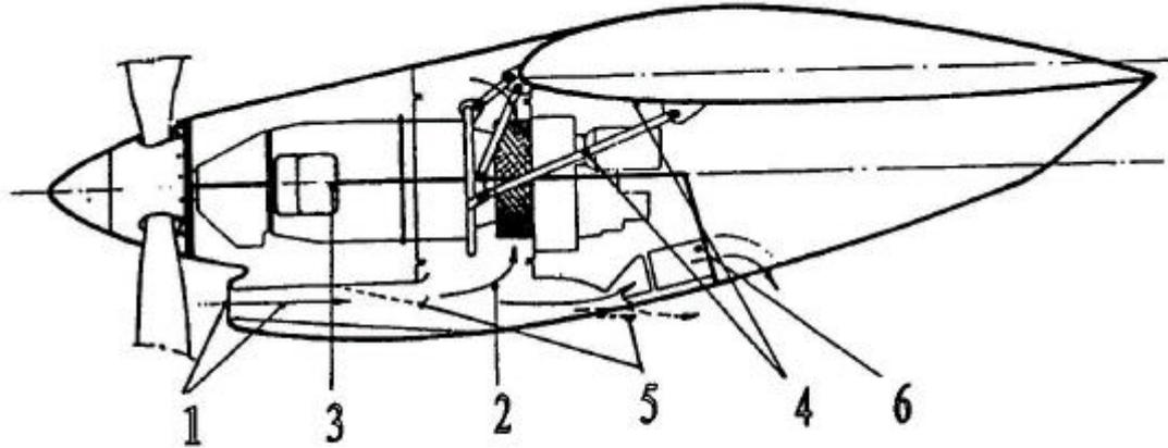
Condition for mounting the engine to the airframe structure can be met by using the engine B 061 001N mount ring, which is supplied together with the engine (the aerobatic M601T engine is supplied with the EM601.95-815 mount ring). If this mount ring is not used it is necessary to the installation must be consulted with WALTER a.s. producer. An aircraft with PT6 engine is easily rebuilding to M601 by using the M601-164.6 engine mount ring.
