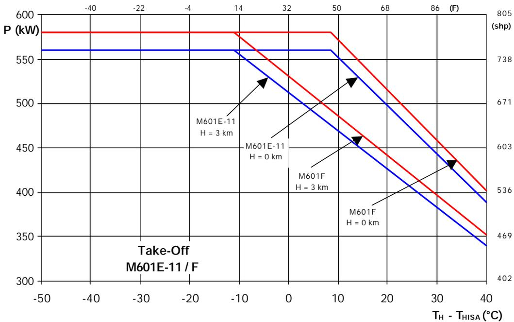
$T_{HISA} = 15\text{ }^\circ\text{C}$  (59 F) at alt.  $H = 0\text{ km}$  ;  $T_{HISA} = -4.5\text{ }^\circ\text{C}$  (29.3 F) at alt.  $H = 3\text{ km}$  (914.4 ft)
