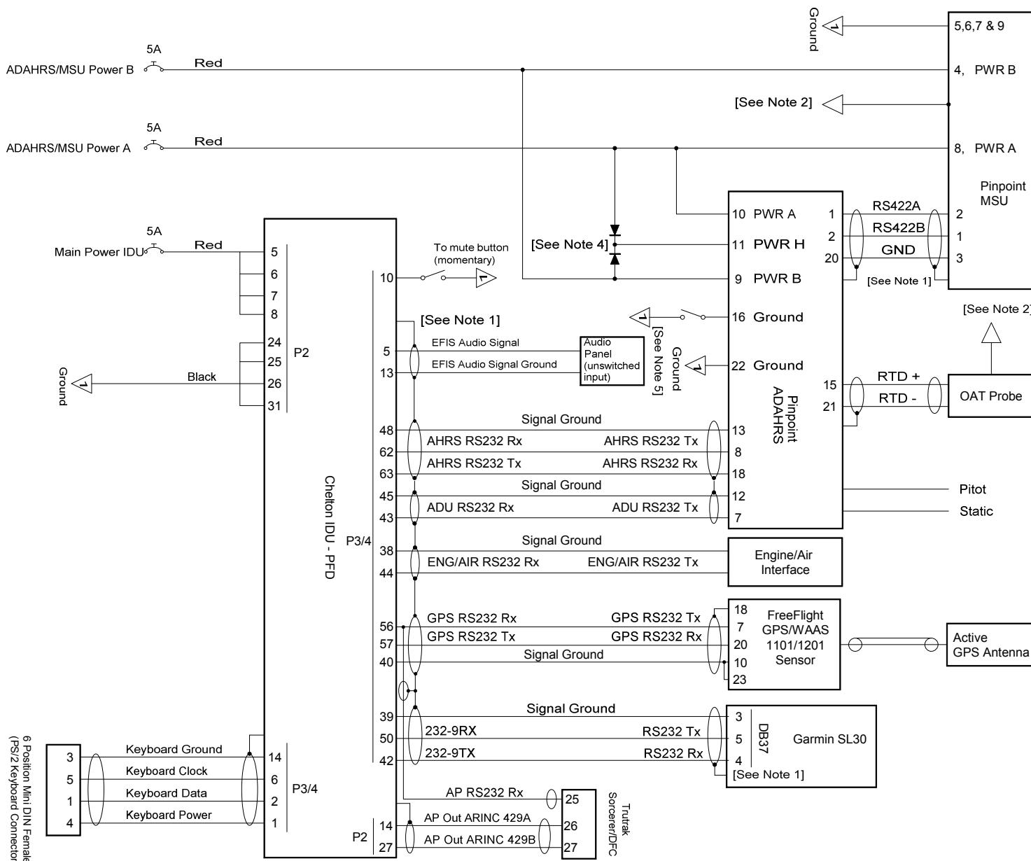
Connector on the ADAHRS is MS38999, 22Pin
