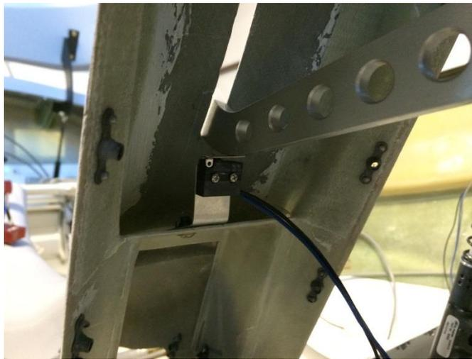
Canopy latching lever micro switch mounting example
