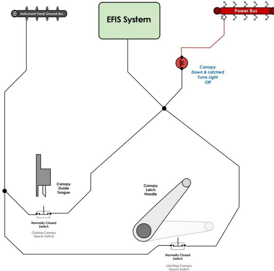
Canopy Safety Wiring Drawing Example
