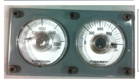
After parking a cold soaked plane in a warm hangar: The Low side pressure has risen to 1,200 psi. Note the High side circuit is unaffected.
