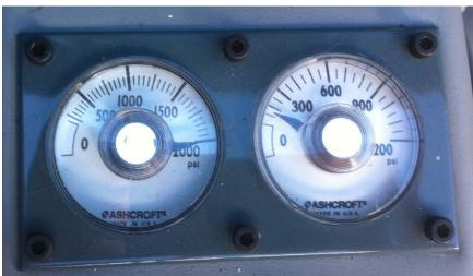
After descent from high altitude: Warmer conditions below have caused the High side pressure to rise. Note that the Low side is unaffected.
