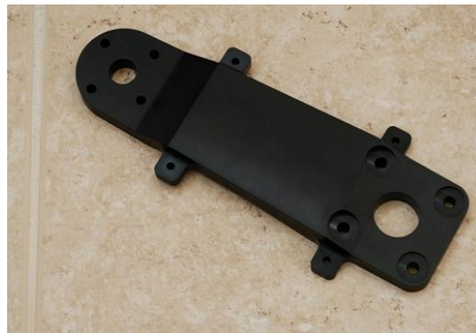
Figure 4, New Trailing with Gear Door Attachments
