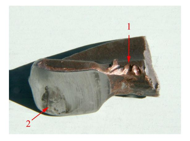
Figure 7 Gouges (arrow 1) and wear on the rocker tip surface (arrow 2).
