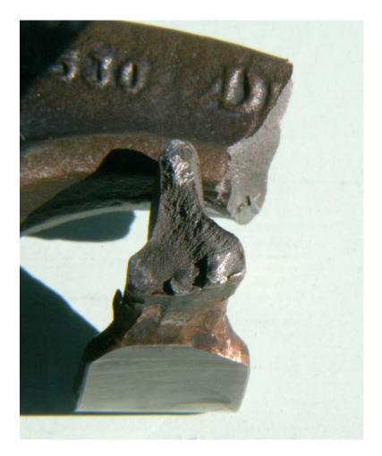
Figure 2 Fracture surfaces on the detached rocker tip and main arm. The curved rocker tip surface is bright and free from copper. Original grinding scores from manufacture can be seen on the rocker tip
