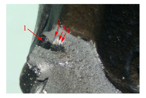
Figure 12 Magnified view of the multiple secondary origins of fatigue. Arrow 1 indicates a dark area of casting seam. Arrow 2, arrow 3 and arrow 4 indicate jogs which are a characteristic feature of multiple origin fatigue. The jogs are long thin triangular steps formed where fatigue cracks on slightly different planes approach each other and the ligament of metal breaks between the two fatigue cracks.
