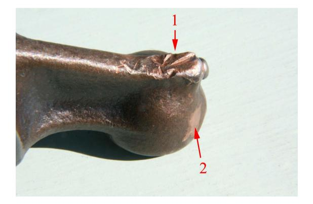
Figure 10 Indentations (1) on the top surface of the push rod cup housing. Arrow 2 indicates an area of polishing wear on the outside surface of the cup housing.
