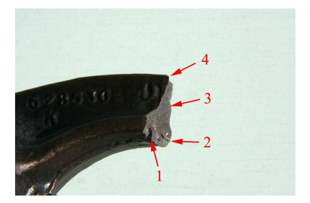
Figure 3 Oblique view of features evident on the main arm fracture surface. Arrow 1 indicates a dark area in an axial plane. Arrow 2 indicates smearing metal on the fracture surface. Arrow 3 indicates the main fracture surface. Arrow 4 indicates a shear lip.
