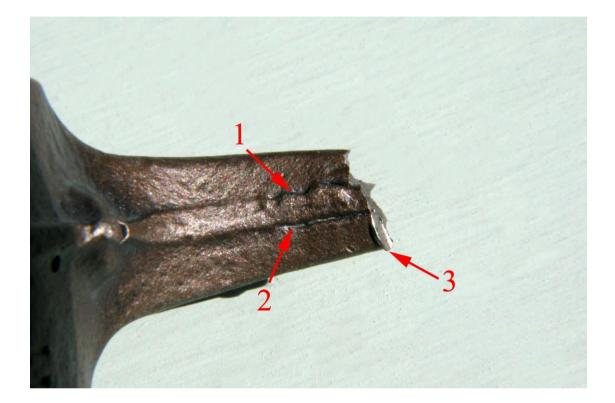
Figure 5 Underside of the broken rocker arm. Arrow 1 and arrow 2 indicate the grooves to either side of the mould joint line. Arrow 3 indicates a flow lip associated with the area of smeared metal on the fracture surface.
