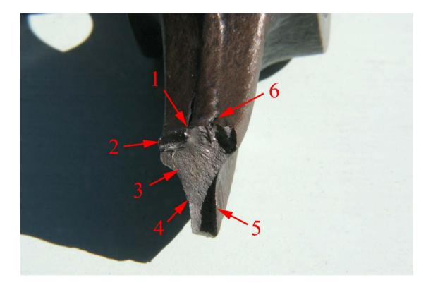
Figure 4 Main arm fracture surface viewed inverted and in the axial direction. Arrow 1 indicates an axial groove along one side of a mould joint line. Arrow 2 indicates the region of smeared metal. Arrow 3 indicates a lightly tarnished area containing fatigue crack growth striations. Arrow 4 indicates the transition between lightly tarnished and brighter fracture surface. Arrow 5 indicates the shear lip. Arrow 6 indicates another axial groove along the other side of the mould joint line.
