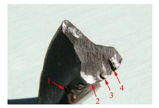
Figure 6 Fracture surface on the detached piece of rocker tip. Arrow 1 indicates a set of gouges. Arrow 2 indicates an area of polishing on the fracture surface. Arrow 3 and arrow 4 indicate surfaces which correspond to extensions of the two grooves shown in figure 5.
