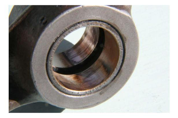
Figure 8 Polishing wear of the bearing bushes.
