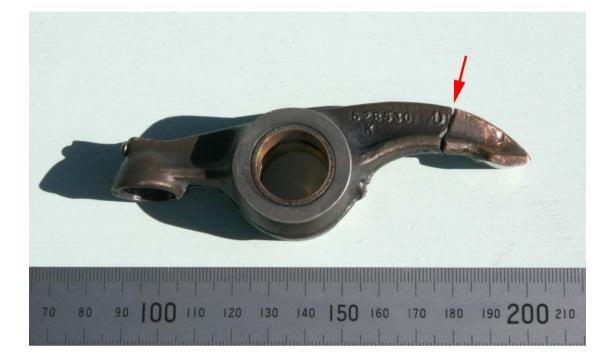
Figure 1 General view of the broken rocker arm with the fracture position indicated by an arrow. The embossed casting identification is 628530 K ADI. The colour indicates that the rocker arm was electroplated with copper during manufacture.
