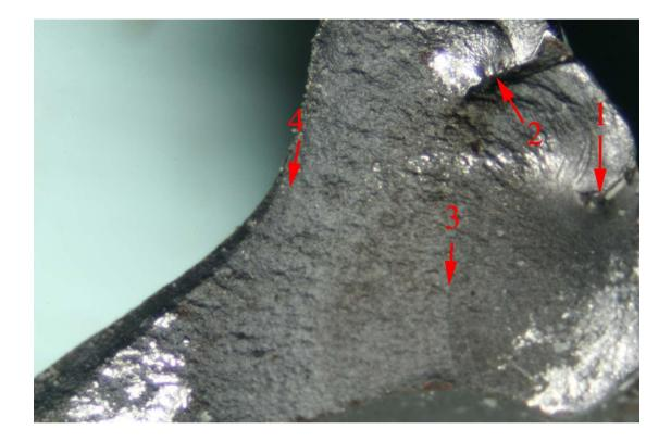
Figure 11 Magnified view of part of the fracture surface on the detached piece of rocker arm tip. Arrow 1 indicates an origin of fatigue at a seam in the casting. Arrow 2 indicates multiple origins of fatigue on a second seam in the casting. This region appears to have been a secondary origin of fatigue. Arrow 3 indicates one of the more distinct fatigue crack arrest striations. Arrow 4 indicates fainter and more widely spaced fatigue crack arrest striations.
