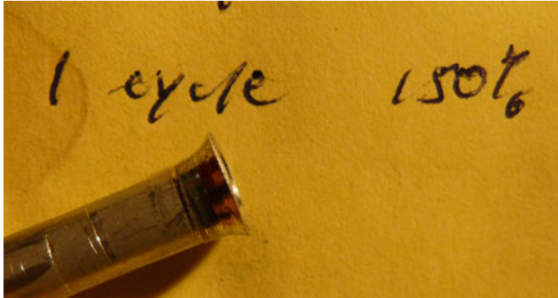
Tube flare after one cycle at 150% of recommended torque
