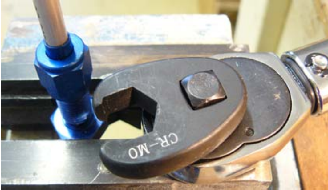
Three-eighths drive torque wrench with crow foot to drive AN 818 nut
