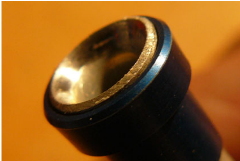
New tube flare, never used, with proper tube flare length
