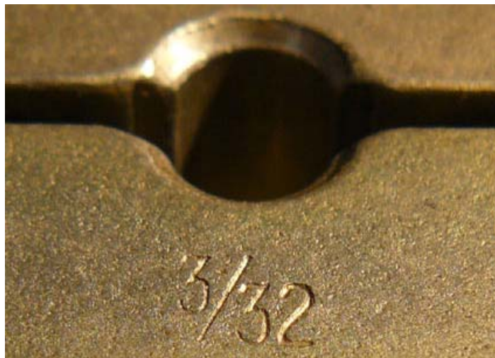
Tube clamp that holds tubing during flaring process
