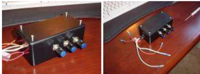
I used Velcro to install the controller box behind the drivers seat.
