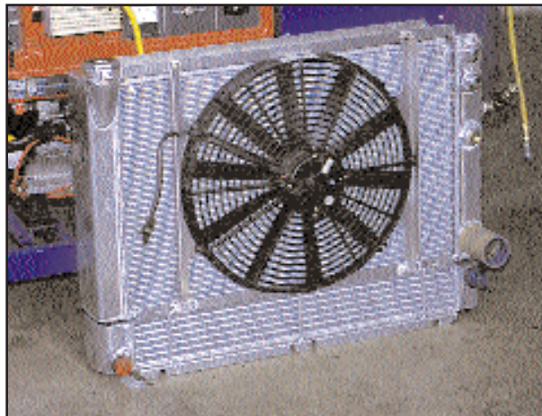
NASCAR radiators are constructed of welded aluminum and range from 3-1/2” to 7”, depending on the type of track being raced on.
